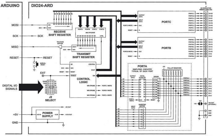
Figure 1 - DIO24-ARD Block Diagram
