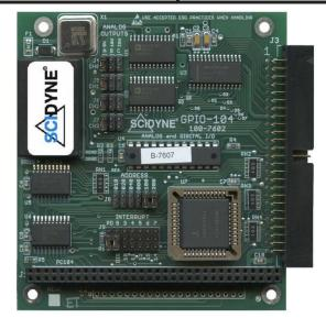
The GPIO-104 is an 8-bit analog and digital input/output module designed to satisfy a broad range of applications. Its generous assortment of functions and capabilities will, in many instances, make the GPIO-104 the only peripheral module required. It conforms to the PC/104 (IEEE-996.1) standard, operates on a single +5V power supply, and uses a single 50-Position IDC header for all I/O connections.
