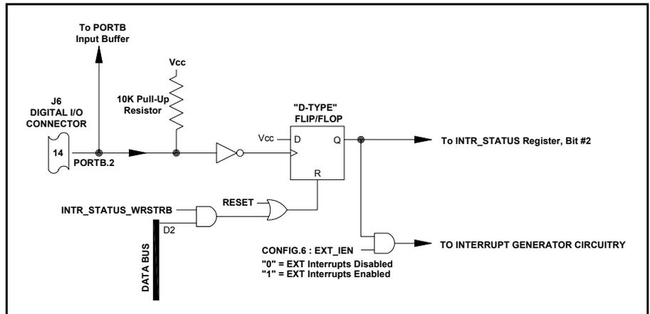
Figure 10 - External Interrupt Circuitry Block Diagram
