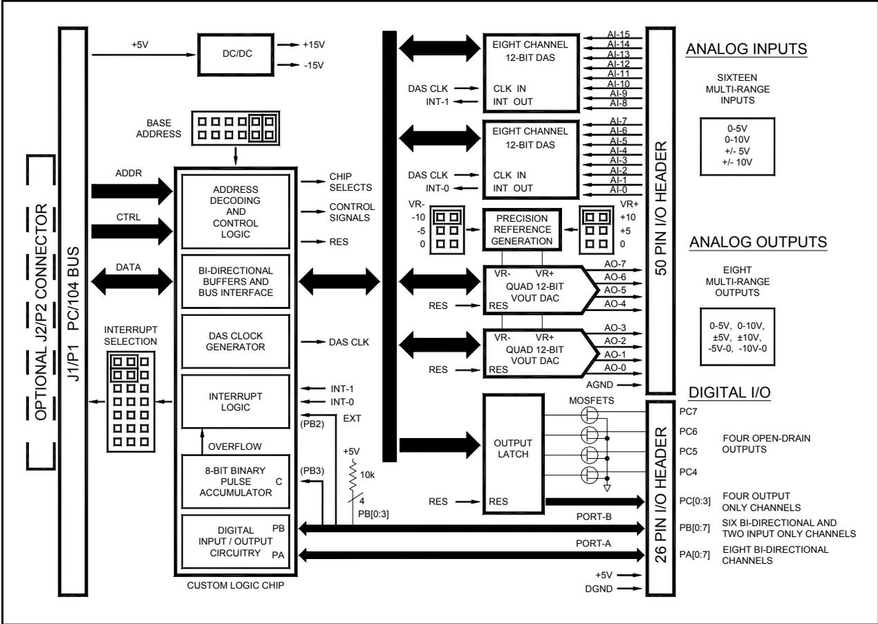
Figure 1 - ADIO Block Diagram
