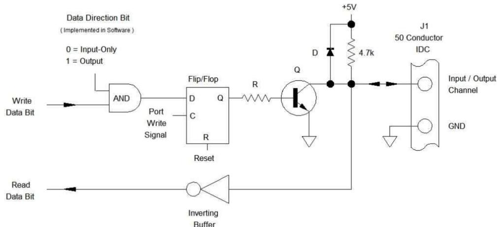
**Figure 4 - Simplified I/O Channel Circuitry**
