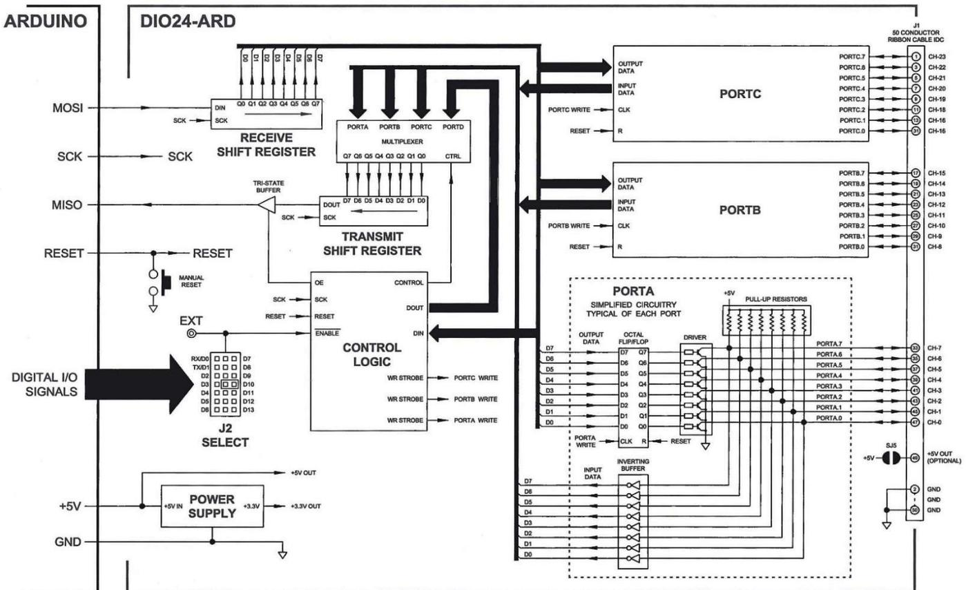
Figure 1 - DIO24-ARD Block Diagram
