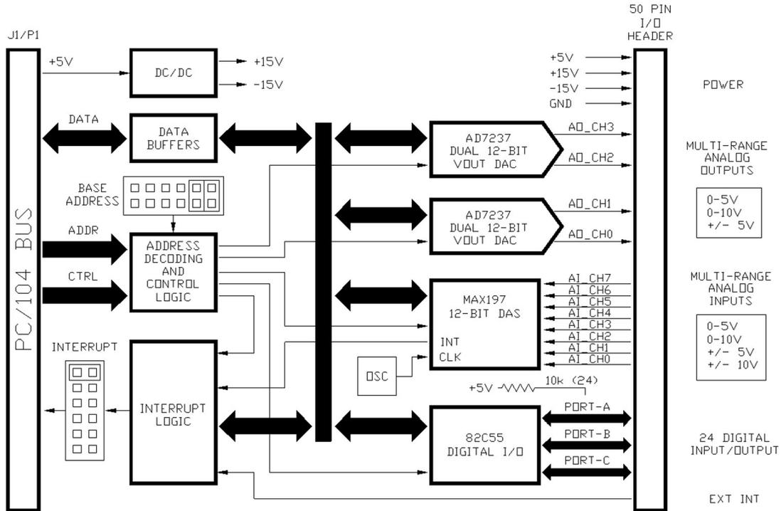
Figure 1 – GPIO-104 Simplified Block Diagram
