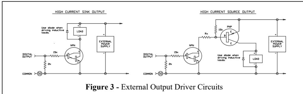
Figure 3 - External Output Driver Circuits
